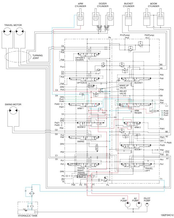
When the left control lever is pulled back, the arm spools in the main control valve are moved to the arm in position by the pilot oil pressure from the remote control valve.
