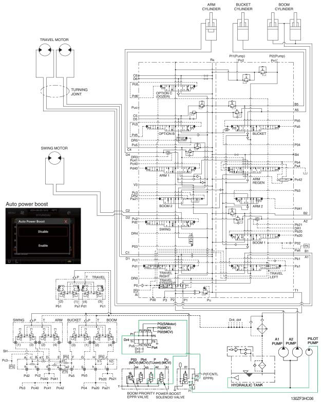
When the power boost switch on the left control lever is pushed ON, the power boost solenoid valve is actuated, the discharged oil from the pilot pump flows into **Pu** port of the main relief valve of main control valve; then the setting pressure of the main relief valve is raised from 330 kgf/cm<sup>2</sup> (4690 psi) to 360 kgf/cm<sup>2</sup> (5120 psi) for increasing the digging power.
