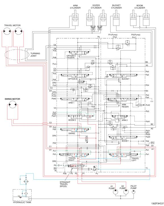
When the swing and travel functions are operated simultaneously, the swing spool and travel spools in the main control valve are moved to the functional position by the pilot oil pressure from the remote control valve and straight travel spool is pushed to the right by the pilot oil pressure from the pilot pump.
