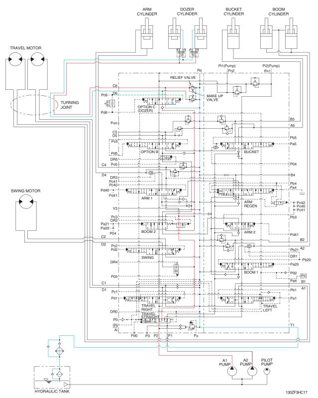
When the dozer control lever is pushed forward, the dozer spool in the main control valve is moved to the dozer down position by the pilot oil pressure from the remote control valve.
