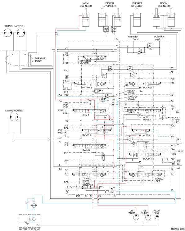
When the left control lever is pushed forward, the arm spools in the main control valve are moved to the arm out position by the pilot oil pressure from the remote control valve.
