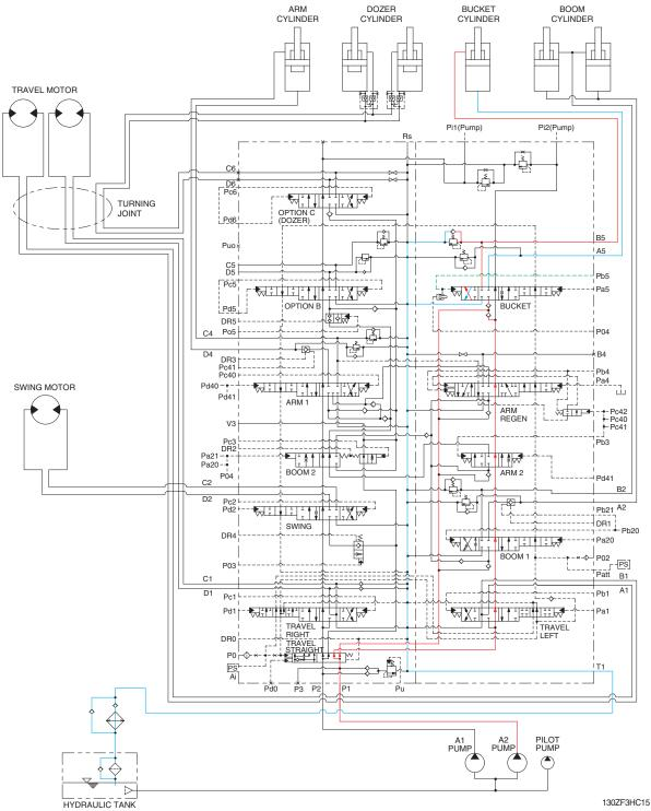
When the right control lever is pushed right, the bucket spool in the main control valve is moved to the bucket out position by the pilot oil pressure from the remote control valve.
