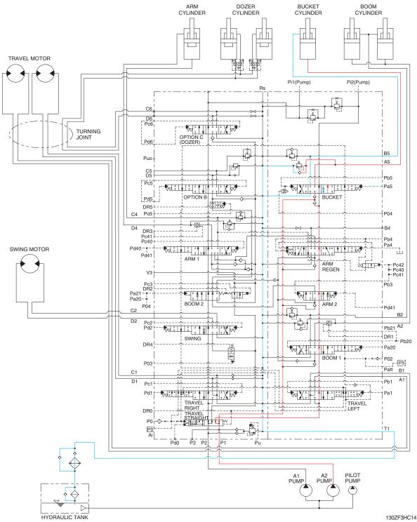
When the right control lever is pulled left, the bucket spool in the main control valve is moved to the roll in position by the pilot oil pressure from the remote control valve.
